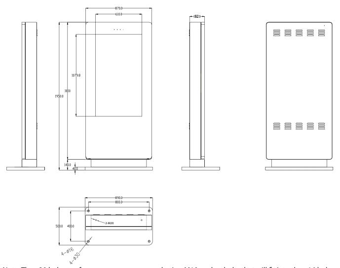
Note: The  $\emptyset 30$  holes are for access, we recommend using M10 anchor bolts that will fit into the  $\emptyset 16$  holes.
